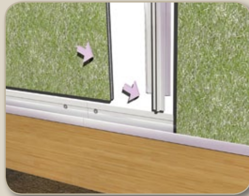
2. Using adhesive, install the Panels and select one of the many Reveal options for a beautiful vertical detail
