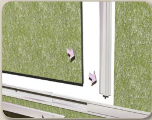
4. Continue the installation by adding Panels and Reveal Hardware and Trim
